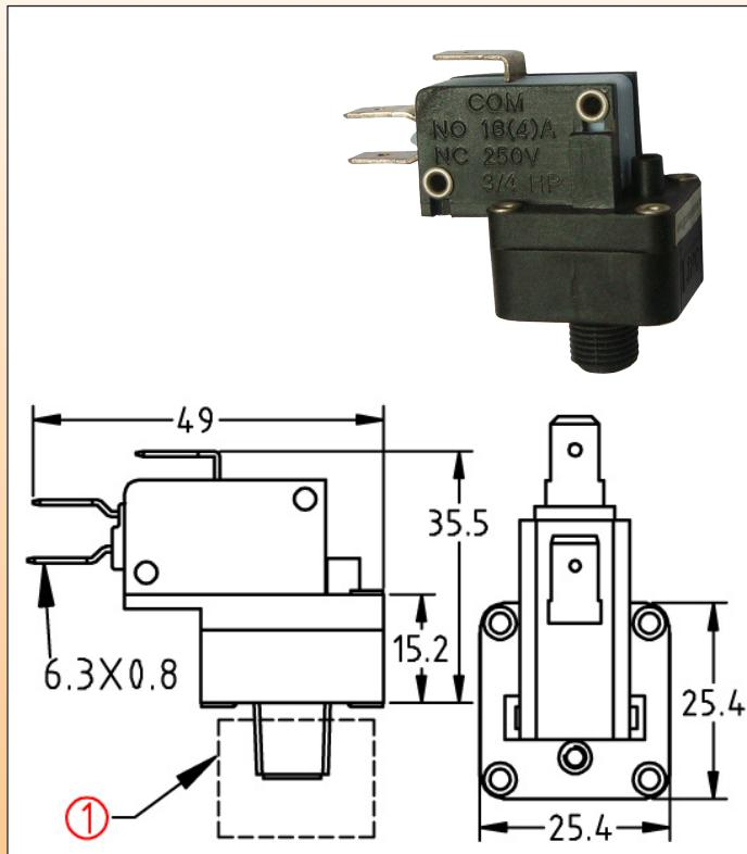
**Uses:** High electrical rating, for 250V.
